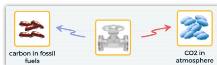
Figure 3b. Semantic representation of flow using nodes and directed links. The flow node has a negative impact on the source collector (blue arrow) and a positive impact on the destination collector (red arrow).
