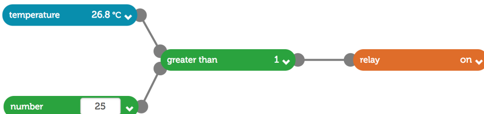
Figure 1. A Dataflow program to turn on a relay when the temperature is above 25 degrees.
