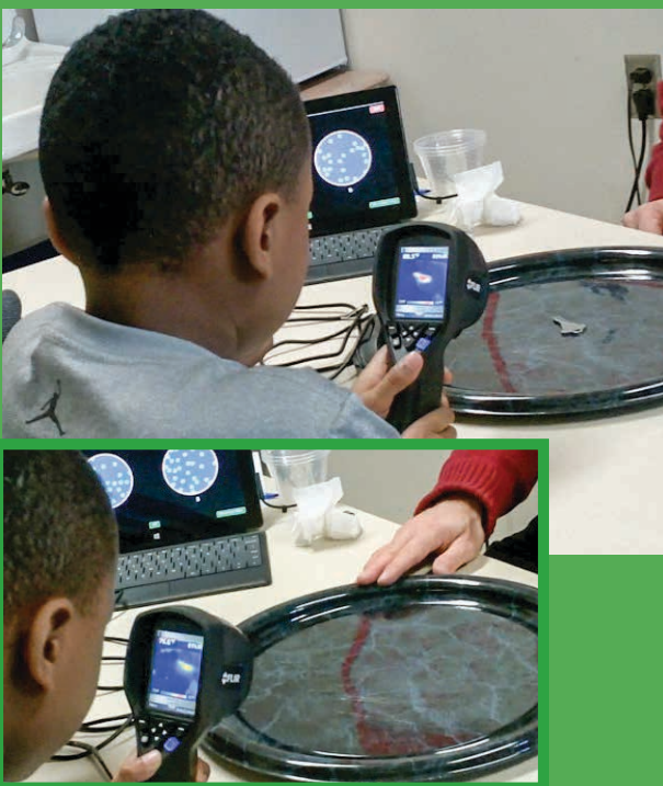
Figure 2. A child views a hot metal key with an IR camera. Inset: A thermal image of the key remains visible after the key is removed.
