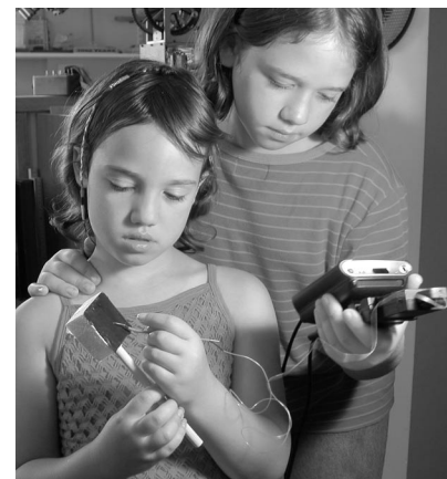
Figure 3. Students hold the black surface of the radiant lollipop near an incandescent lamp to measure heat rise due to absorbed radiation.
