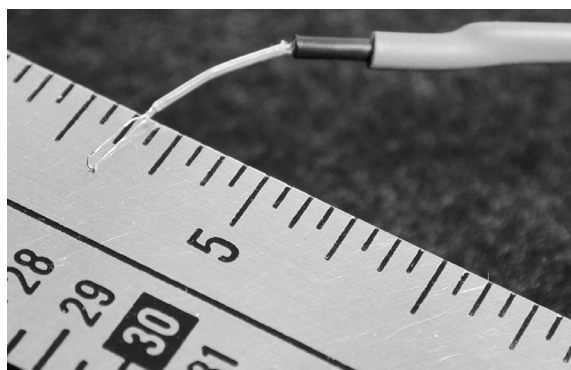
Figure 1. In order to support continuing investigation into heat and temperature, we developed an ultra-fast response temperature probe. The sensing element is the very tiny bulb in the wire that is touching the ruler.
