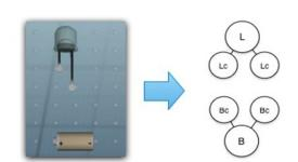
Figure 2. Circuit elements and corresponding topology
